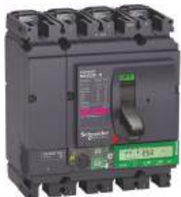
Fig. F78 Exemple of 250 A MCCB with earth leakage measurement and alarming (Compact NSX Micrologic Vigi 4.3)
