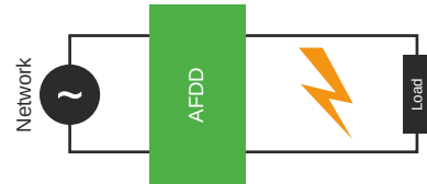
Fig. F81 Parallel arc fault
