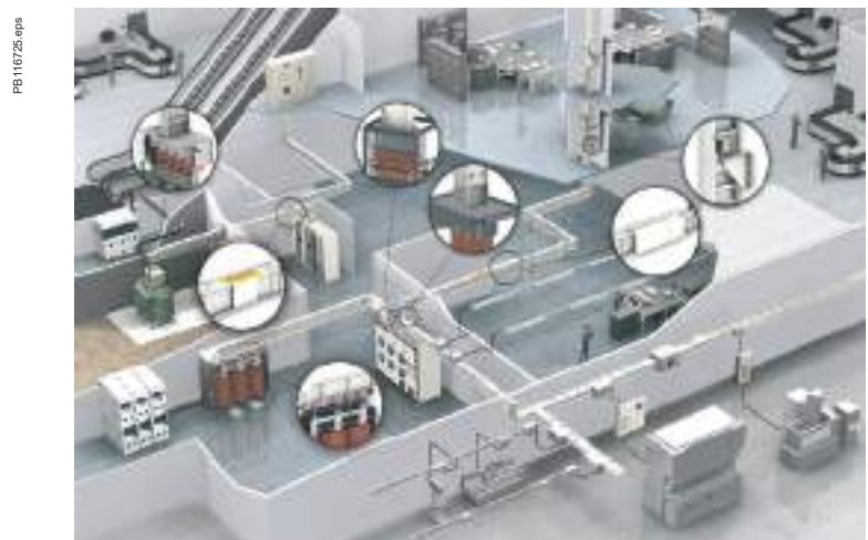
Fig. E45 Radial distribution using busways
