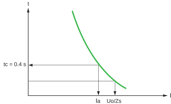
Fig. F21 Disconnection by fuses for a TN system
