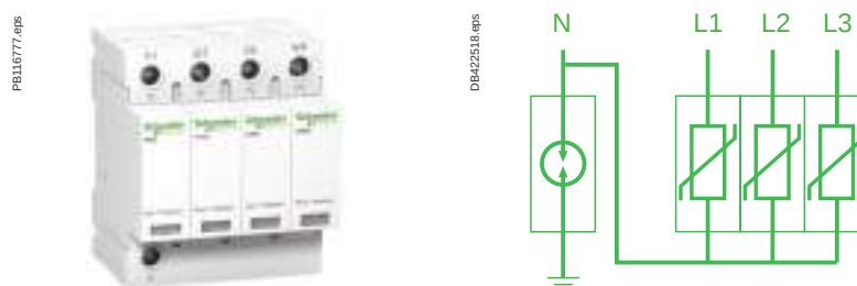
Fig. J52 The Schneider Electric brand iPRD SPD incorporates a gas discharge tube between neutral and earth and varistors between phase and neutral
