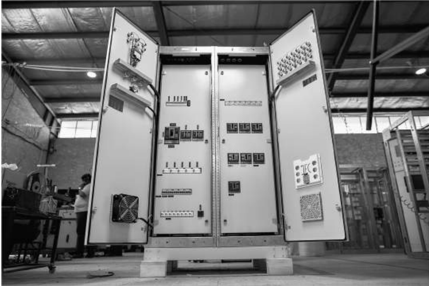
LV/ LIGHTING PANEL 0.4 KV CCS TYPE
